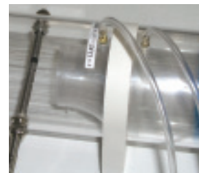
Measuring across the nozzle for air velocities between 3,0... 12 m/s
