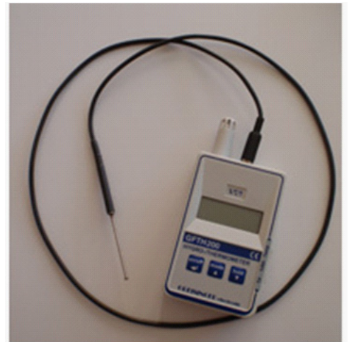
GFTH 200 with extern temperature probe Pt1000
