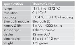
Please note: Bluetooth LE thermometers have a range of 50 metres depending on the users smart device make and model. Environmental conditions may also affect the signal strength.
