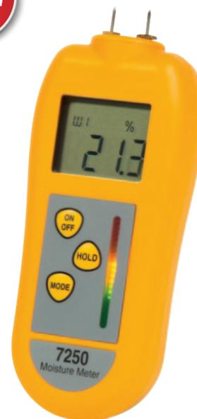
The unit is housed in a robust ABS case and is powered by three AAA batteries that give a minimum of 350 hours battery life. The instrument will power off automatically after ten minutes, maximising battery life. This feature can be disabled by the user, if required.
