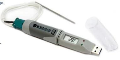
This standalone data logger measures and stores up to 32,510 temperature readings from either a K, J or T type thermocouple. A thermocouple is attached via the thermocouple socket at the base of the unit. The user can easily set up the logging rate and start-time, and download the stored data by plugging the data logger into a PC's USB port and running the purpose designed software under Windows 2000, XP, Vista or 7. Data can then be graphed, printed and exported to other applications.
