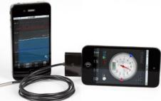
The iCelsius Pro uses a 4" stainless steel tip to report temperature readings through the iPad when the probe is in thermal contact with matter.
