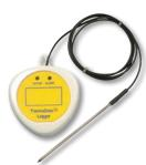
This logger incorporates both an internal and external NTC thermistor probe with a one metre PVC/PFA lead that measures over the range of -40 to 85 °C (internal) and -40 to 125 °C (external) and can record up to 2 x 2000 readings.
