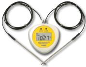
This logger incorporates two external fixed NTC thermistor probes with two one metre PVC/PFA leads that measure over the range of -40 to 125 °C and can record up to 2 x 2000 readings.
