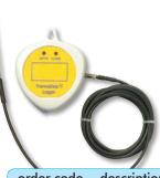
This logger incorporates an external NTC thermistor sensor with a one metre PUR/PVC lead and probe connector that measures over the range of -40 to 125 °C and can record up to 4000 readings.
