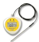
This logger incorporates an external NTC thermistor probe with a one metre PVC/PFA lead that measures over the range of -40 to 125 °C and can record up to 4000 readings.
