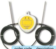
This logger incorporates two external NTC thermistor sensors with two one metre PUR/PVC leads and probe connectors that measure over the range of -40 to 125 °C and can record up to 2 x 2000 readings.
