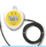
This logger incorporates an external NTC thermistor sensor with a one metre PUR/PVC lead and probe connector that measures over the range of -40 to 125 °C and can record up to 4000 readings.
