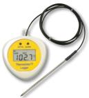
This logger incorporates both an internal and external NTC thermistor probe with a one metre PVC/PFA lead that measures over the range of -30 to 85 °C (internal) and -40 to 125 °C (external) and can record up to 2 x 2000 readings.
