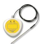
This logger incorporates an external NTC thermistor probe with a one metre PVC/PFA lead that measures over the range of -40 to 125 °C and can record up to 4000 readings.
