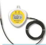
This logger incorporates both an internal and external NTC thermistor sensor with a one metre PUR/PVC lead and probe connector that measures over the range of -40 to 125 °C and can record up to 2 x 2000 readings.
