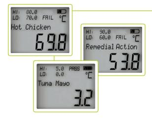
With the checklist items loaded onto the handheld, readings are stored with location, user, date, time and limits. Up to 1000 readings are stored before upload is required. Attach the appropriate type K thermocouple probe and store readings with the press of a button. Scroll quickly through your checklist with the  $\blacktriangle \blacktriangledown$  buttons.
