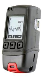
This stand-alone data logger measures and stores over 250,000 temperature readings over a -30 to  $+80^{\circ}$ C (-22 to  $+176^{\circ}$ F) range at a resolution of 0.1°C
